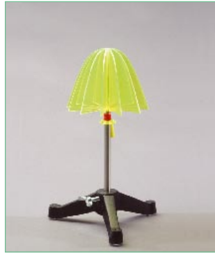
15 Rotationsmodell eines Paraboloids. Sechs von Parabeln begrenzte Flächen. Rotation model of a paraboloid. Six surface elements delimited by parabolas rotate about their axis of symmetry.
