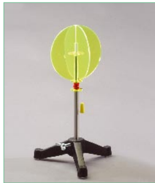
688 Rotationsmodell zur Kugel- entstehung, zur Demonstration der Guldinschen Regel. Rotation model for generating a sphere to demonstrate the theorem of Pappus (or Guldin).
