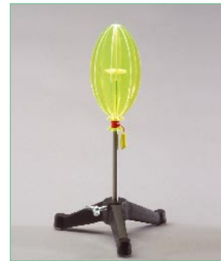
690 Rotationsmodell für ein gestreck- tes Ellipsoid, zur Demonstration der Guldinschen Regel. Prolate ellipsoid (or spheroid) of rotation to demonstrate the theorem of Pappus (or Guldin). Four ellipses rotate about their major axis of symmetry.
